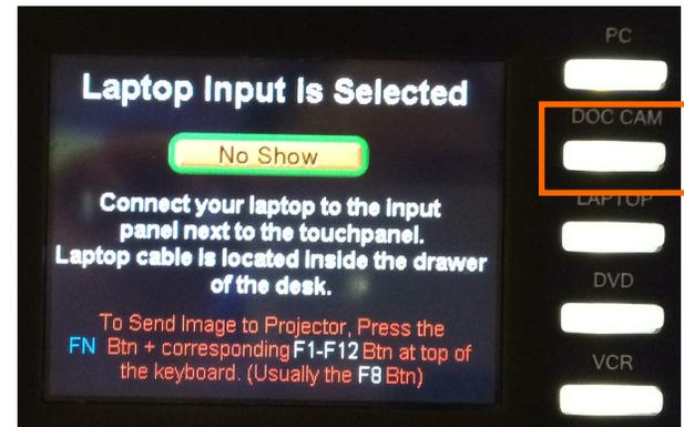
8. **LAPTOP**- Changes the source to **Laptop**. Note: VGA and Audio cables to connect Laptop to control panel are located in the multimedia desk drawer. If VGA/Audio cables are not in the desk, call the IT Help Desk and press 3 to connect to AV/Classroom Support.
