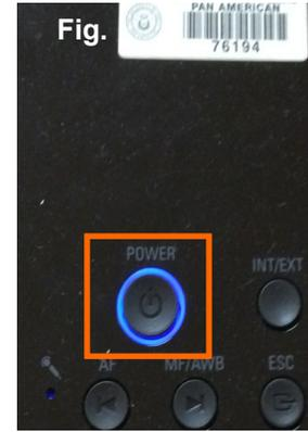
Press the **Power** button to turn document camera on (Fig. 7). Wait a few seconds for Document Camera (**Doc Cam**) to warm up. Press **Power** button again to turn off Doc Cam.
